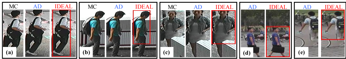
Figure 1.7: Comparisons of person bounding boxes by manually cropping (MC), automatically detecting (AD), and identity discriminative attention reinforcement learning (IDEAL). Often AD contains more background clutter (a,d,e). Both AD and MC may suffer from occlusion (c), or a lack of identity discriminative attention selection (b).
