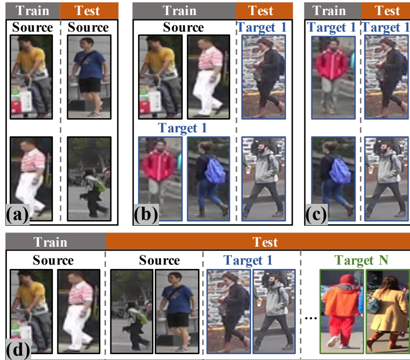
Figure 1.9: Learning strategies for person re-id: (a) Supervised model learning on a large set of cross-camera identity labelled training data per domain. Once trained, the model is deployed for the same domain alone. (b) Unsupervised domain adaptation on labelled training data from a source domain and unlabelled training data from the target domain. The adapted model is specific for the target domain. (c) Unsupervised model learning on unlabelled training data of the target domain. The trained model is specific for the target domain. (d) Universal model learning on labelled training samples from a source domain. Once trained the model can be frozen forever and applied for universal person re-id deployment at any target domains including the source domain. (Source Domain: Market-1501 dataset [43]; Target 1 Domain: DukeMTMC dataset [59]; Target N Domain: MSMT-17 dataset [41] )
