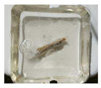
Figure 2.6: Ballistic gel with embedded bone.
