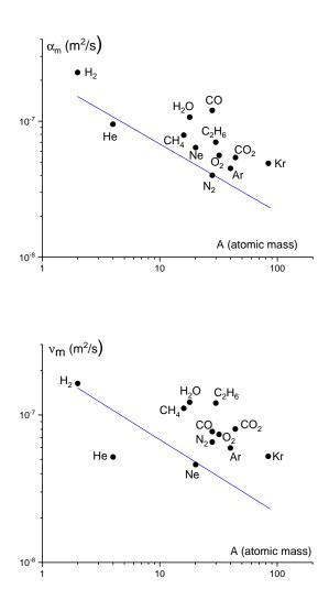
FIG. 3. Points show experimental  $\alpha_m$  (top) and  $\nu_m$  (bottom) as a function of molecular mass. The solid line is the prediction of Eq. (11).
