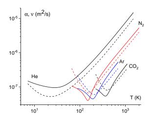
FIG. 2. Experimental  $\alpha$  (solid lines) and  $\nu$  (dashed lines) for He (20 MPa), N<sub>2</sub> (10 MPa), Ar (20 MPa) and CO<sub>2</sub> (30 MPa) [22].
