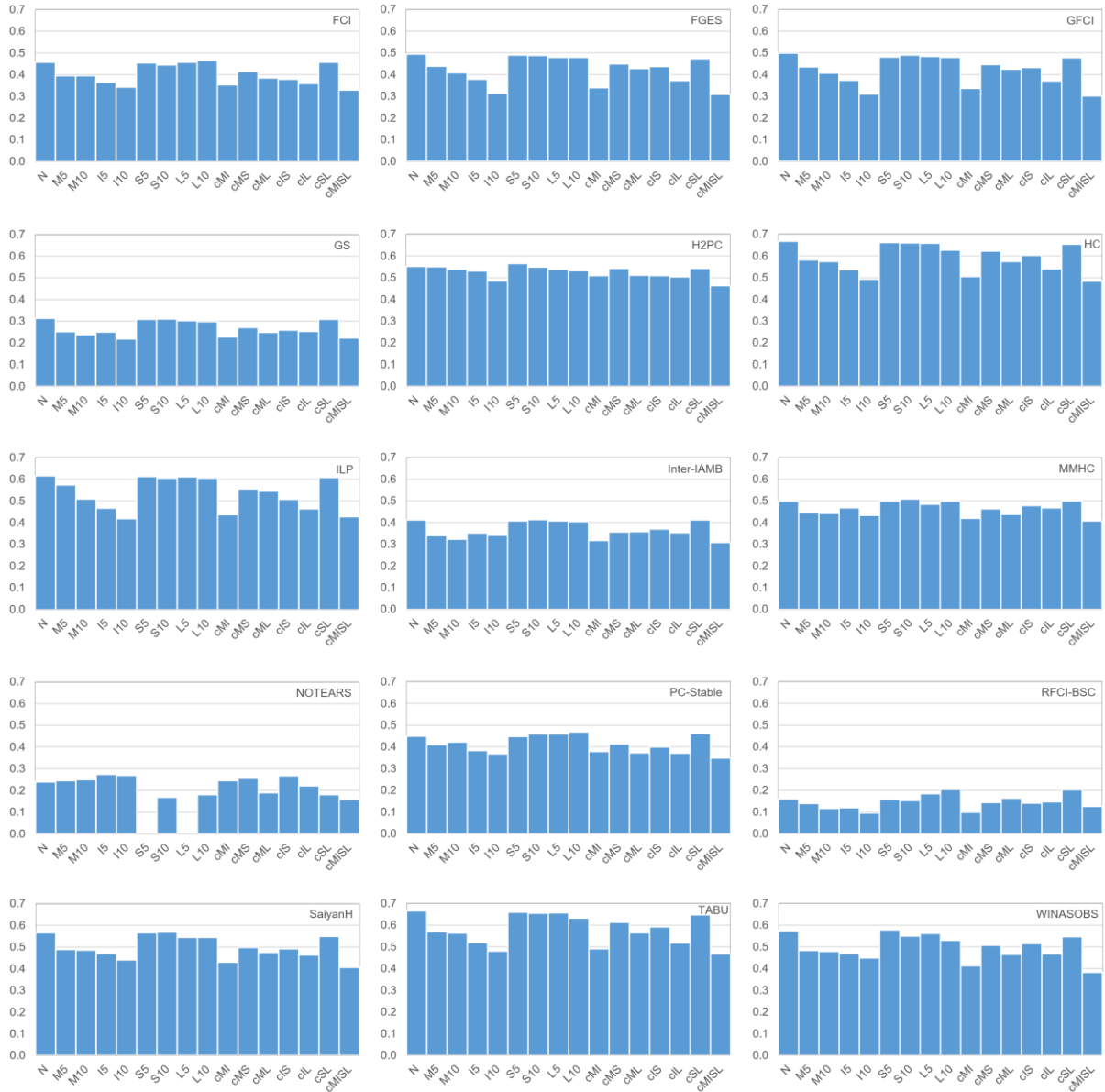
Fig 8. The impact different types of data noise ( x -axis) have on the combined average score \frac{(F1+BSF)}{2} ( y -axis) of the algorithms across all sample sizes and case studies. Because some of the average scores depicted in these graphs contain missing scores due to failures by some algorithms to produce a graph (refer to Appendix C), these graphs are only useful for determining the relative performance across data noise experiments, and not between algorithms.
