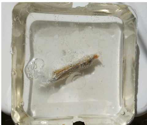
Figure 6: Ballistic gel with bone embedded.
