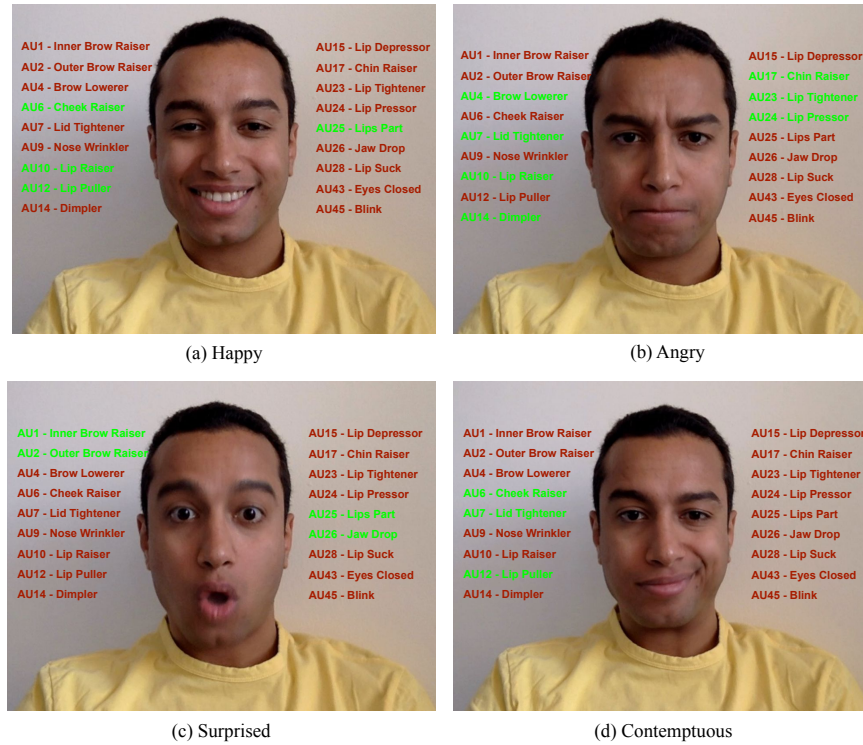
Figure 3.5: Results obtained by the proposed method on some videos. The 18 detected AUs are shown on the processed frames. If any of the AUs are detected, the associated text turns into green, otherwise its colour stays red.
