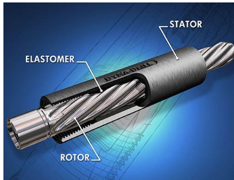
Figure 25: A diagram of a mud motor including the metal rotor and cross section of the elastomer stator
