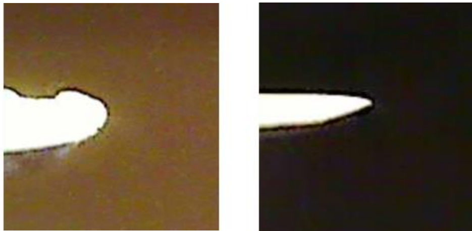
Figure 88: Crack tip shapes for HNBR 0 (left) and HNBR 75 (right) during cyclic pure shear tests at the same strain
