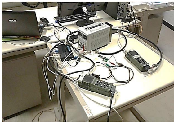
FIGURE 2.4: SDR testbed in the SHIELD project to generate wideband spectrum measurements: hardware platform
