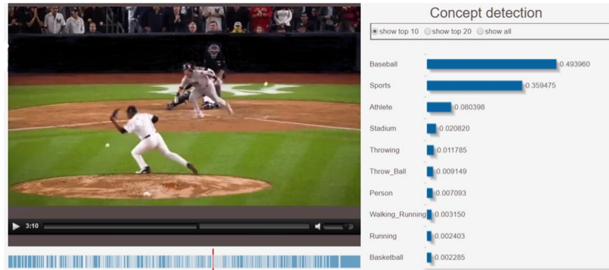
Fig. 1.9: Visual inspection of the results of our DCNN trained model, when applied on a specific video (downloaded from YouTube); here we are considering the concept-based keyframe annotation problem, i.e. whether we can annotate a given keyframe with the most relevant concepts.
