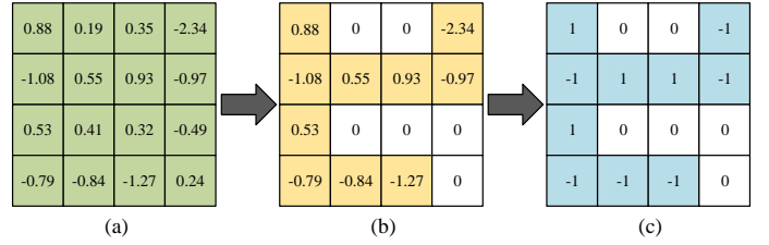
Fig. 4. Flowchart of the proposed joint pruning-quantization, (a) the original weights matrix; (b) the weights after pruning, where the example pruning function is x = 0 for x < 0.5 ; (c) the weights after quantization, where the example quantization function is x = \text{sign}(x) .
