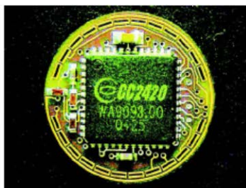
(b) Top view of the fabricated transceiver layer
