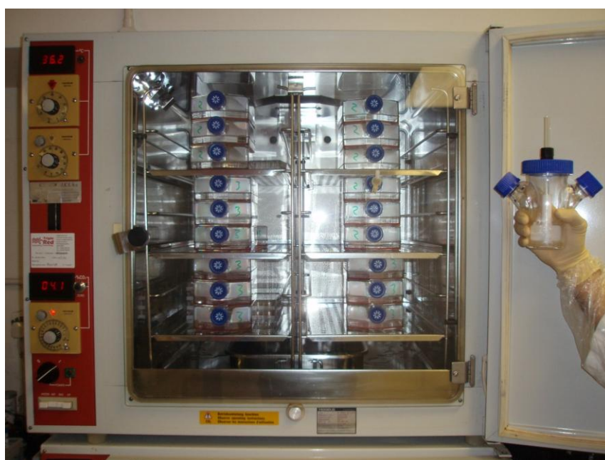
Figure 13: The surface area of microcarriers within the spinner flask on the right is equivalent to the surface area of the T-flasks within the incubator.
