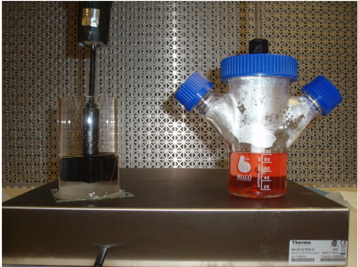
Figure 41: PIV replica (left) and the spinner flask (right).
