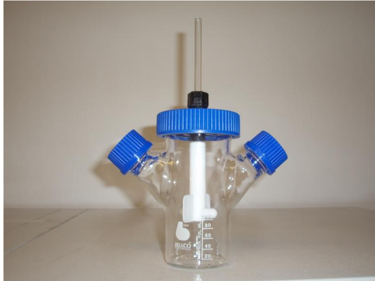
Figure 6: Spinner Flask manufactured by Bellco Glass Inc (USA). It is used specifically for microcarrier culture and has a working volume of up to 100 ml. The impeller is coloured white and has a magnet attached to it. A magnetic stirrer is used to rotate the impeller.
