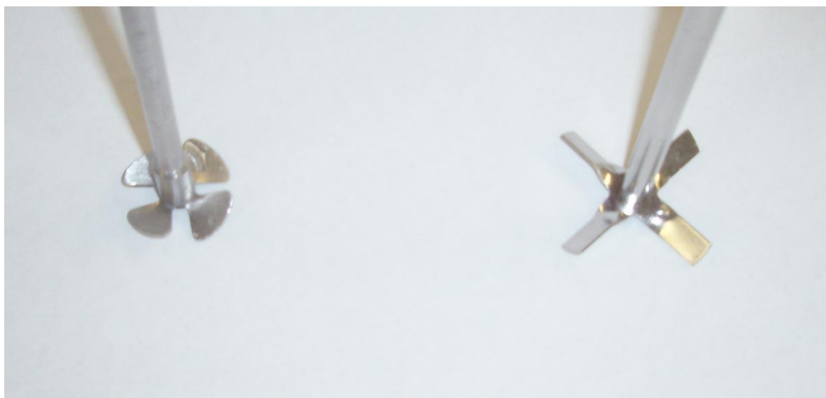
Figure 30: Propeller-design impeller (30 mm diameter) on the left-hand side for the production of smoother PCL microcarrier surfaces. Pitch-blade impeller (49 mm diameter) on the right-hand side for the production of rougher PCL microcarrier surfaces.
