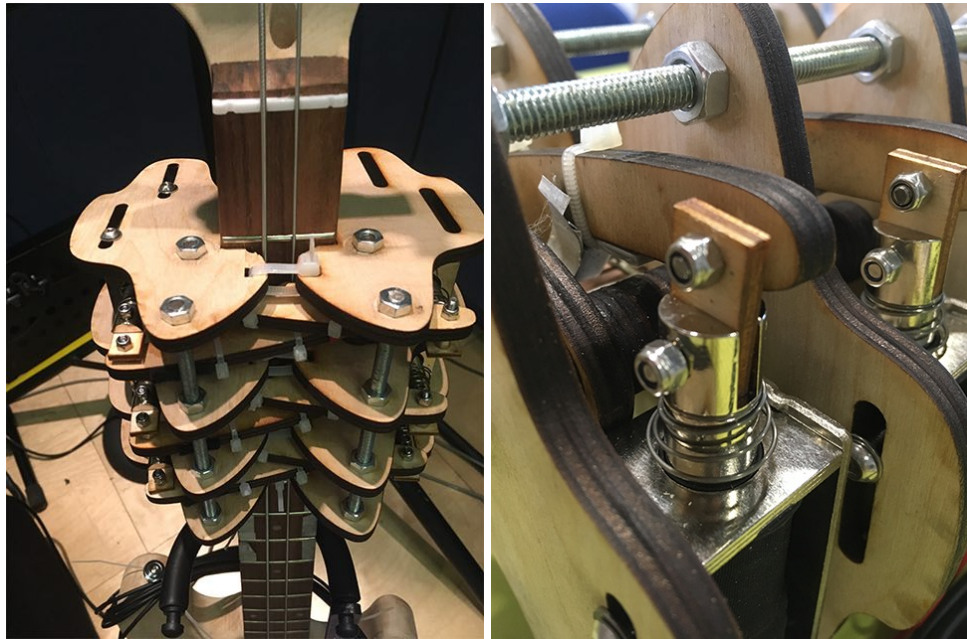
Figure 4.5: a) side view of neck clamp; b) solenoid plunger attachment to tip of fretting arm
