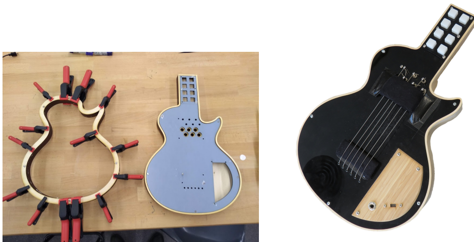
Figure 6.3: L: build process of S2 instrument using layers of glued plywood. R: finished S2 instrument
