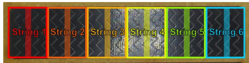
Figure 5.7: Trill sensor divided into six string areas
