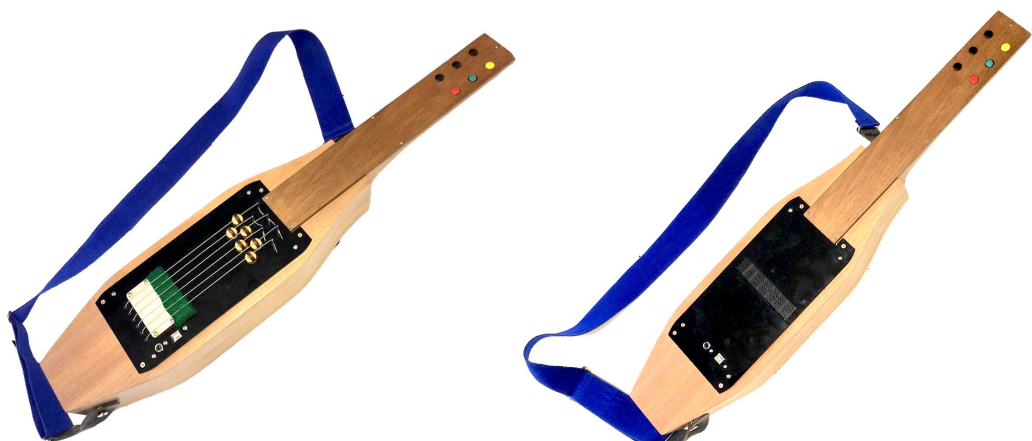
Figure 5.11: The guitar body enclosure with the strings sensor module (SG, left) and touch sensor module (TG, right) inserted
