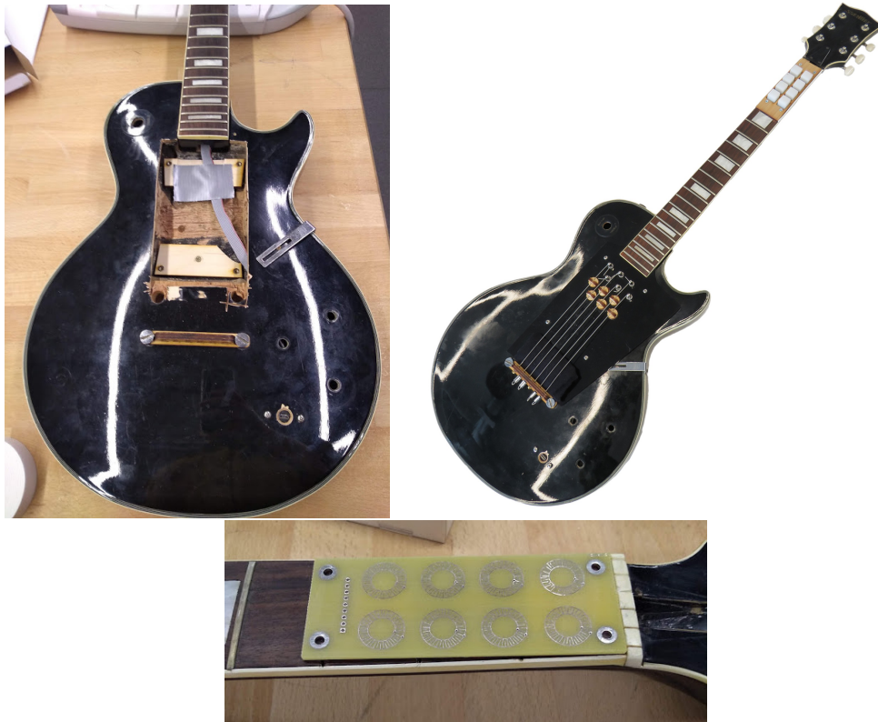
Figure 6.4: L: Les Paul body with material removed for electronics. R: completed S3 instrument. Bottom: custom PCB made to fit neck width
