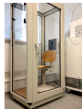
Ventilated chamber with carbon filter attached to ventilation unit in addition to HEPA filter
