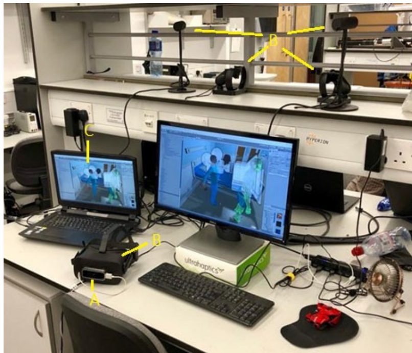
Fig. 6. Hardware configuration to run the auscultation training simulator. A) The Leap Motion. B) The Head Mounted Display with its controllers and tracking stations. C) A VR ready laptop.
