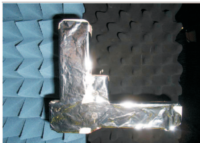
Figure 3.2: The metallic foil wrapped MDF gun replica
