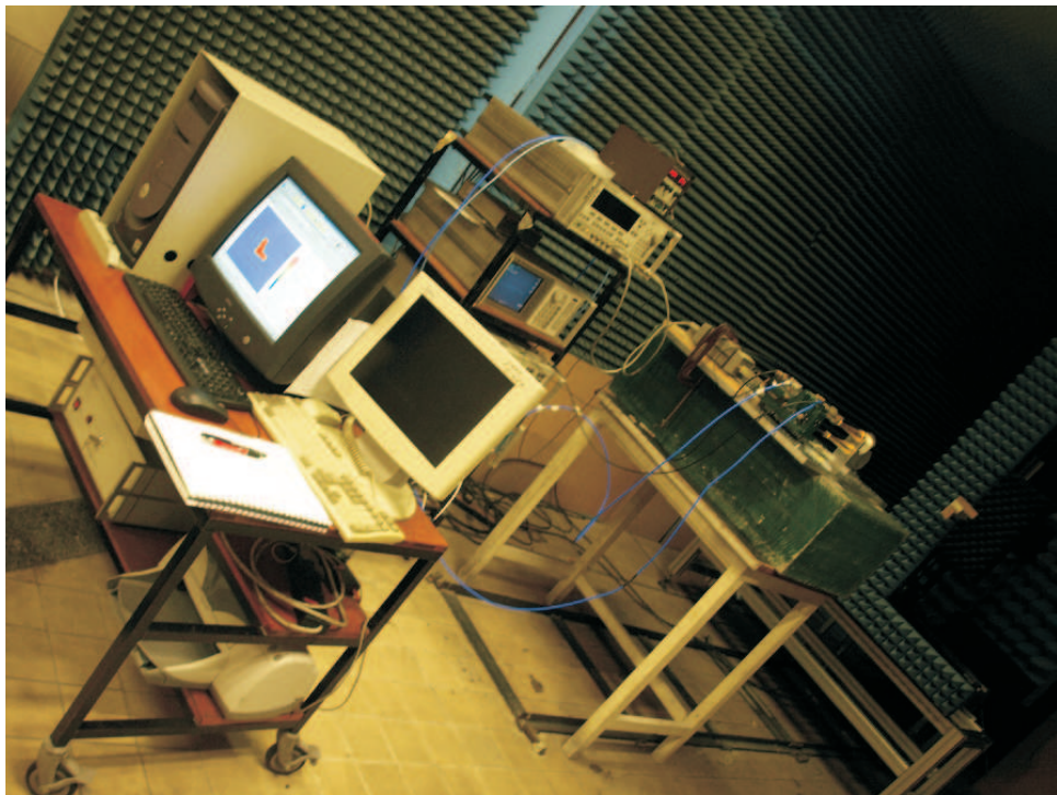
Figure 2.7: Photograph of the 94 GHz microwave holographic imager
