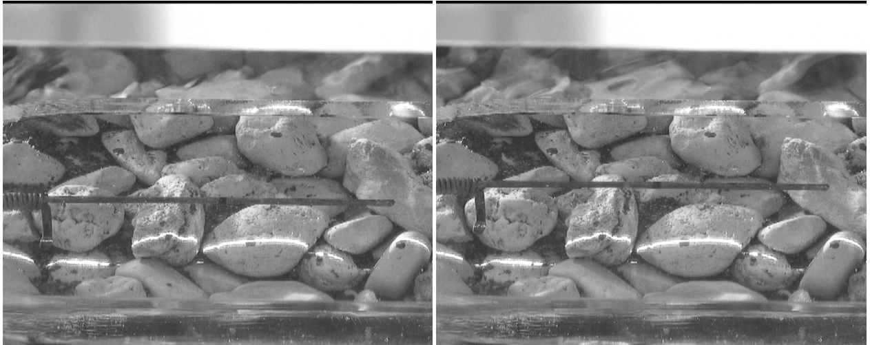
Fig. 3. The calibration rod (104 mm long) moved from position 1 (left) to position 2 (right) by a \Delta y = 10 mm.
