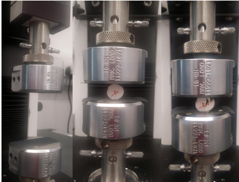
Figure 9: Brazilian diametral test using the Instron machine with two flat metal plates covered by sand paper for a better grip. The picture demonstrates a typical disc failure
