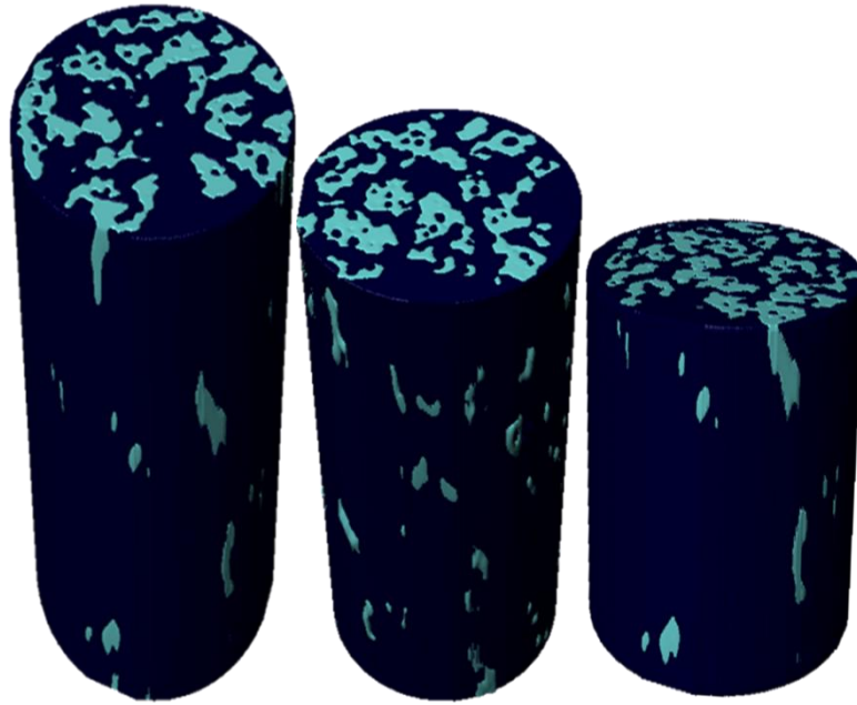
Figure 32: Volume rendered RVEs with dual masks to determine conservation of porosity after cutting to shorter cylinders. The RVEs created for the 7020 porous hydroxyapatite. The light blue mask for the hydroxyapatite material and the dark blue mask for the empty space (porosity)
