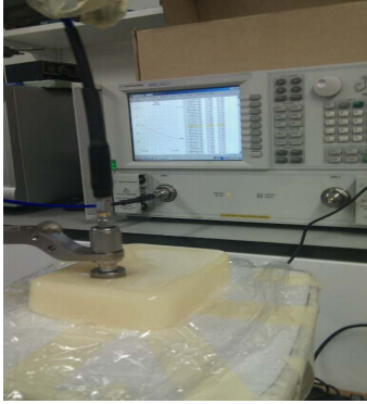
Fig. 1. Dielectric property measurement set-up with Agilent's high temperature dielectric probe.
