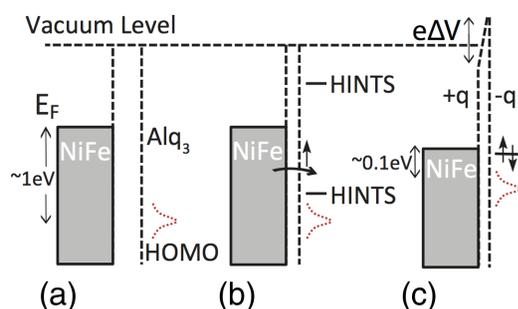
FIG. 1. Energy diagrams showing the decrease of hole injection barrier due to the presence of HINTS in the first molecular layer of Alq<sub>3</sub>, (a) NiFe/Alq<sub>3</sub> energy diagram in separation (no HINTS), (b) the introduction of HINTS and electron transfer, (c) reduction of hole injection barrier due to charge transfer into the occupied HINTS.
