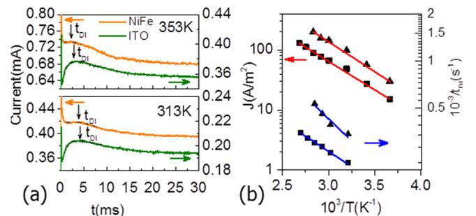
FIG. 3. (a) Typical temperature dependent DI on NiFe-Alq<sub>3</sub> (500nm)-Al and ITO-Alq<sub>3</sub> (500nm)-Al samples and (b) the Arrhenius plots of the current density and the reciprocal of transient time (proportional to mobility) for both samples.
