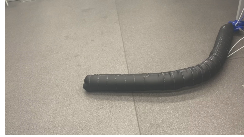
Fig. 1. The soft eversion robot with multiple bending segments.
