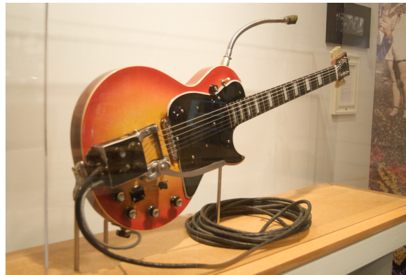
Figure 5. With a black control box (the Les Paulverizer ) mounted on a guitar, Les Paul was able to control tape machines during live performances. Photo © 2010 by Mark Zaputil (Zap Ltd. Music), used with permission.
