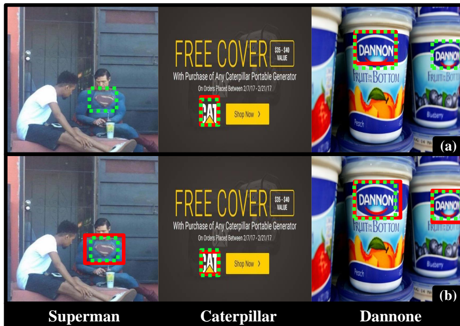
Figure 7: Qualitative evaluations of the (a) WLOD and (b) SL^2 models. Green dashed boxes: ground truth. Red solid boxes: detected. The WLOD fails to detect visually ambiguous (1 st column) logo instance, success on relatively clean (2 nd column) logo instances, while only fires partially on the salient one (3 rd column). The SL^2 model can correctly detect all these logo instances with varying context and appearance quality.
