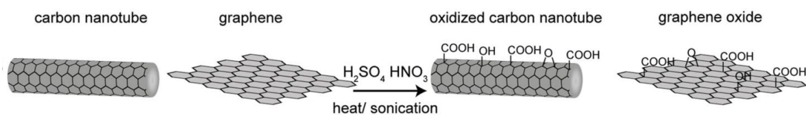
Figure 10: Oxidizing strategies for the introduction of oxygen containing groups for further functionalization of carbon nanostructures. (taken from ref 16).
