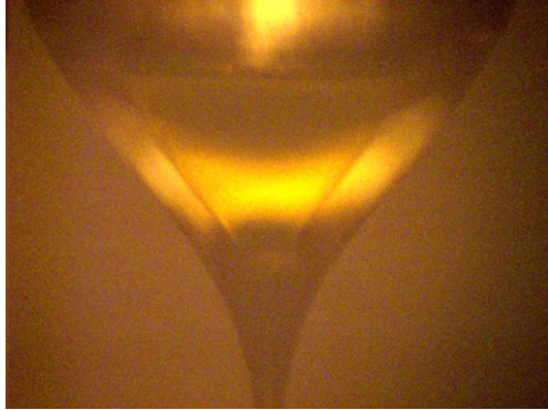
Figure 2.9 Cone-jet mode of coaxial electrospray
