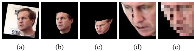
FIGURE 8: Sample images at different stages during the data set generation process. (a) Original image with 250 \times 250 pixels, (b) image after fitting a 3D morphable model at 0^\circ pitch angle, (c) image with synthetic pitch effect produced by applying a 3D geometric transformation, (d) aligned image with 96 \times 96 pixels produced by applying an affine transformation based on the detected eyes and nose locations and (e) down-sampled image emulating an image captured at a different height.
