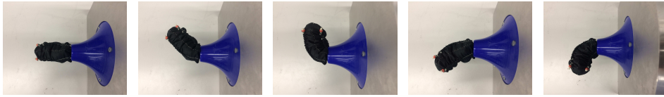
Fig. 2. The manoeuvrability of the soft, inflatable manipulator.
