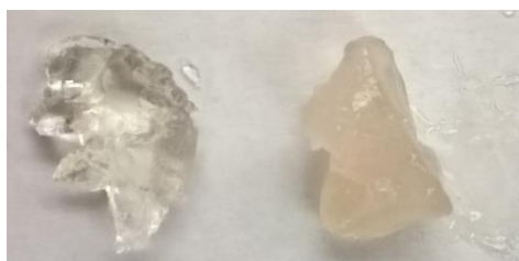
Figure 3.10 Image of CMC gels with a low (20:1 CMC: CaCl 2 ) salt concentration added on the left and a high (1:1) salt concentration on the right. It is clear that at high salt concentration the CMC begins to precipitate out and becomes heterogeneous, hence the cloudy appearance of the gel.
