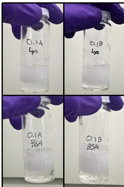
Figure 4.7 Image showing emulsions made using mineral oil and PBS with BSA and Lysozyme as the proteins and benzoyl chloride (marked A) or sebacyl chloride (marked B) as the surfactant. The surfactant was always used at a concentration of 0.1 mg/ml and the protein concentration was kept at 10 mg/ml
