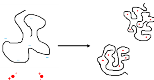
Figure 3.8 Schematic showing the result of the addition of inorganic divalent cationic crosslinks on CMC gels.
