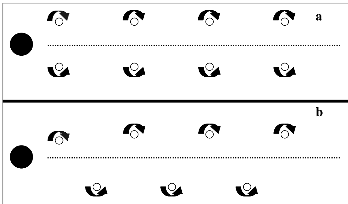
Figure 2.1. Double row of vortices shed from a two-dimensional cylinder (shaded). Flow is from left to right. (a)- symmetric arrangement; (b)- asymmetric arrangement.
