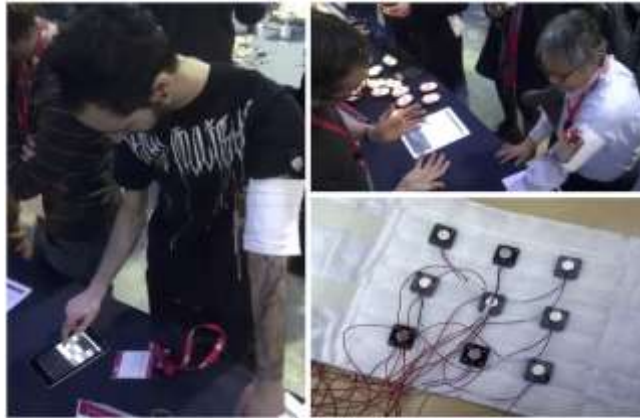
Figure 6: Vibrosign armband prototype and controlled application were tested by visitors in a demonstration session at the Tangible, Embedded and Embodied Interactions conference in 2013 (left and top-right); vibrotactile interface of Vibrosign, showing nine tactors arranged in a 3-by-3 grid display.
