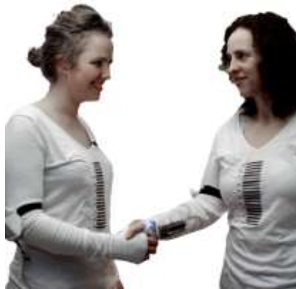
Figure 14: Two volunteers are wearing IBT prototypes, with the peripheral social display inlaid in the frontal area to reveal their compatibility after shaking hands.
