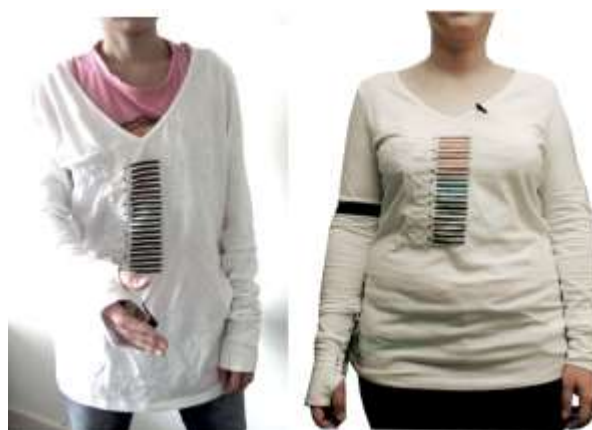
Figure 16: A demonstration of prototypes of IBT, showing the display in idle (left) and subtle notification (right) modes.
