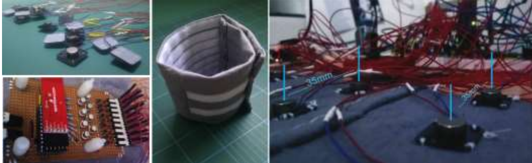
Figure 7: Material and configuration of Vibrotactile armband prototype. Factors (8-by-4.3 mm) mounted on 1-by-100-by-100 mm acrylic supports, with Velcro sheets, to optimise the resonating force on the skin contact area (top left); Vibrosign system circuit (bottom left); an early prototype of armband base with Velcro stripes for experimenting with two-point discrimination threshold (middle); and factors positioned 35 mm apart from the centre-point of each other (right).
