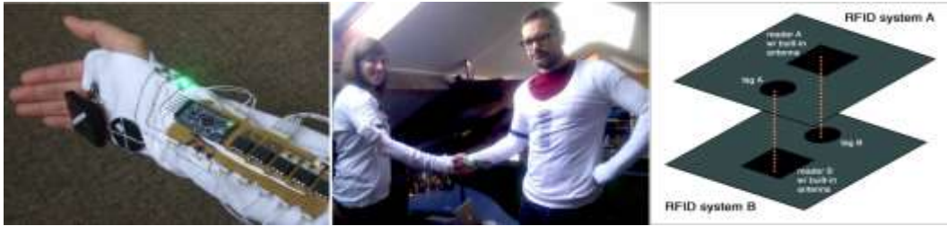
Figure 18: An RFID system consisting of an ID-12 RFID reader and passive 125 kHz RFID tag, embedded on the sleeve-end of IBT prototype and wired to the main circuit controller (ATmega328 IC in Arduino Pro Mini) using conductive threads (left). When two wearers shake hands (centre), an LED glows to indicate an authentication and data-exchange process occurring. During this period, a dense RFID network (right) is formed, and tag-tag, reader-tag and reader-reader collisions are likely to happen.
