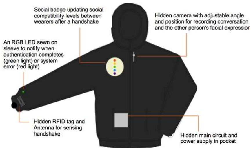
Figure 29: A diagram of Icebreaker Jacket prototype with its features 36
