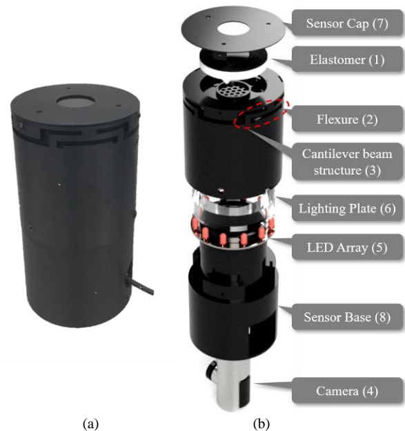
Figure 1. The design of the elastomer-based flexible optical force and tactile sensor: a) manufactured prototype, and b) the design structure.
