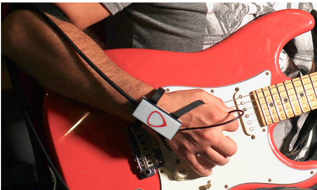
Figure 6: A close up of the wrist box, which contains the preamp board.
