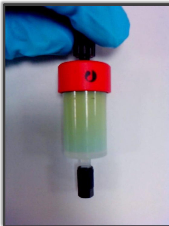
Figure 4.3 Sample of Nfs1 \Delta 1–34 captured on a HisTrap HP affinity column. The protein is bright yellow in colour, a characteristic attributable to bound PLP.
