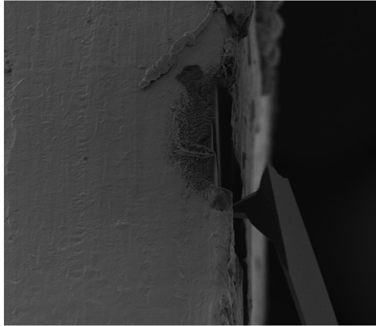
Figure 8.3 SEM micrograph showing the in situ AFM imaging the specimen cross-section
