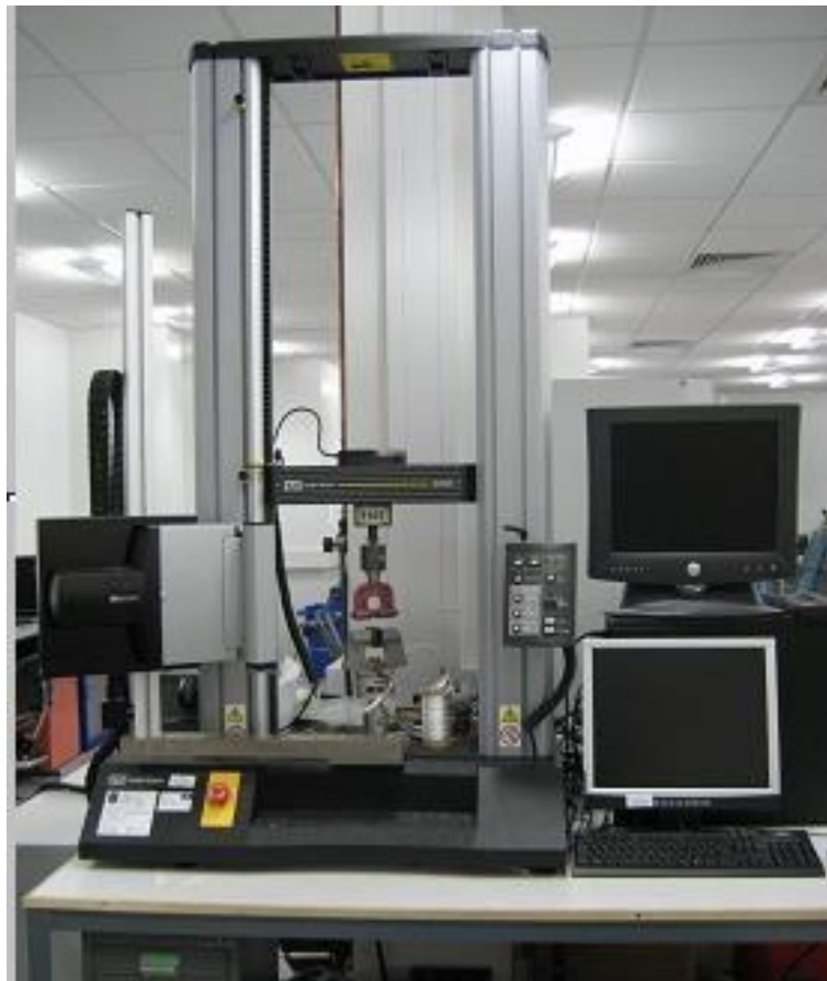
Figure 3.47 Photograph of Instron load frame used to strain polymer nanocomposite samples
