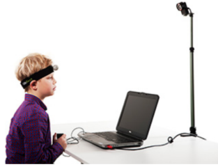
Figure 7.1: The Quantified behaviour Test (QbTest) [129] analyse the head motion to assess attention deficits and hyperactivity.
