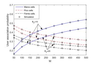
Fig. 2. User association probability versus antenna number with different bias factor, with K = 3, N = 15,  $P_1 = 40$  dBm,  $P_2 = 30$  dBm and  $P_3 = 20$  dBm,  $r_k = 50$  m,  $a_m = 0.6$ ,  $a_n = 0.4$ ,  $\lambda_2 = \lambda_3 = 20 \times \lambda_1$ , and  $B_3 = 20 \times B_2$ .
