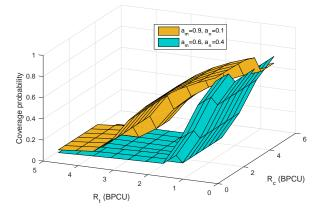
Fig. 4. Successful probability of typical user versus targeted rates of  $R_t$  and  $R_c$ , with K = 2, M = 200, N = 15,  $\lambda_2 = 20 \times \lambda_1$ ,  $r_k = 15$  m,  $B_2 = 5$ ,  $P_1 = 40$  dBm, and  $P_2 = 20$  dBm.
