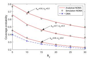
Fig. 3. Coverage probability comparison of NOMA and OMA based small cells. K = 2, M = 200, N = 15,  $\lambda_2 = 20 \times \lambda_1$ ,  $R_t = R_c = 1$  BPCU,  $r_k = 10$  m  $P_1 = 40$  dBm, and  $P_2 = 20$  dBm.
