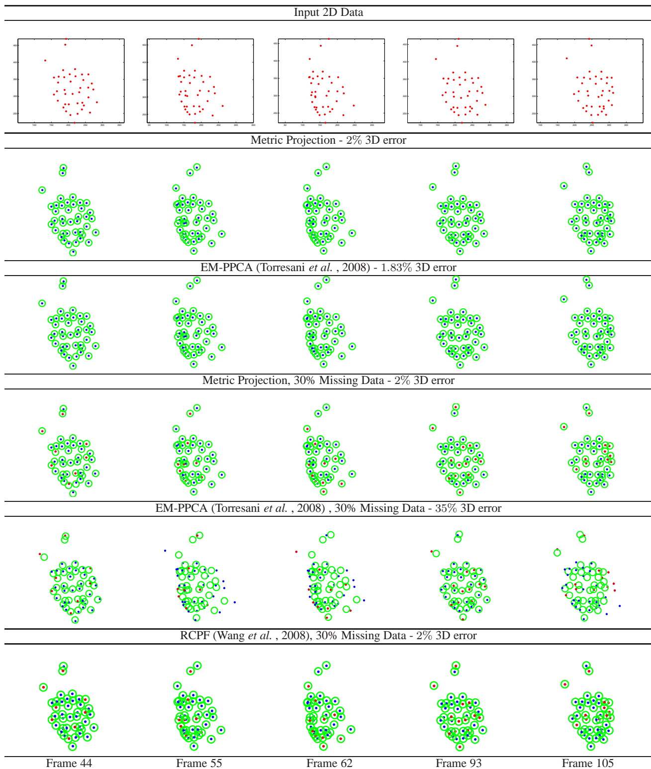
Fig. 5 3D reconstruction results for the “CMU” face motion capture sequence. First row shows the input image data. Second and third rows show the results with full data obtained with our Metric Projection algorithm and Torresani et al. ’s EM-PPCA respectively. The 3D reconstruction results (blue dots) are compared with ground truth data (green circles). Fourth, fifth and sixth rows show comparative results for 30% missing data (missing data points are highlighted in red). Our MP algorithm can recover the 3D shape accurately even with a high percentage of missing data points, while Torresani et al. ’s algorithm gives poor results. The RCPF method also obtains a good reconstruction (2% 3D error) in both cases of full and missing data.
