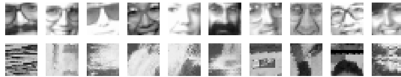
Figure 4.8. Sample SVs of the frontal-view face detector using Gaussian kernel. Top row: positive (faces) SVs, bottom row: negative (nonfaces) SVs.
