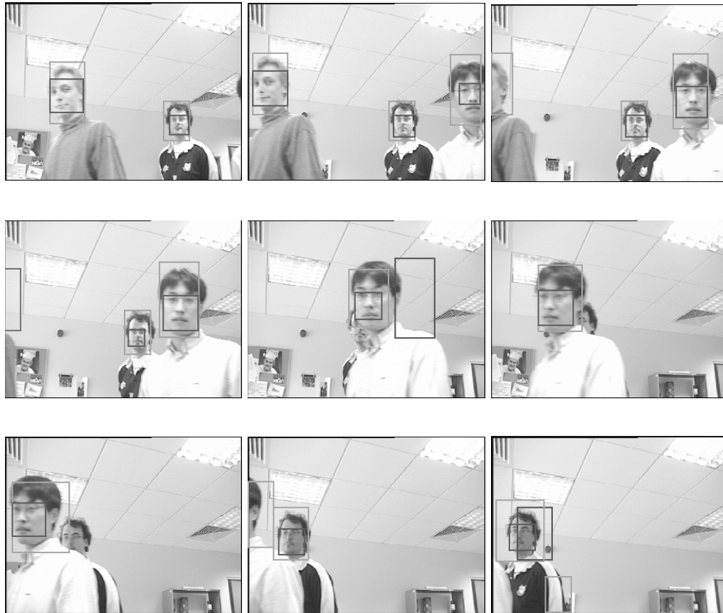
Figure 4.15. Face detection using SVM classifier on a video sequence. The bigger boxes are obtained by motion-colour based selective attention. Face detection is then performed on these bounding boxes only. The final detections are labelled with the smaller boxes inside the bigger ones.
