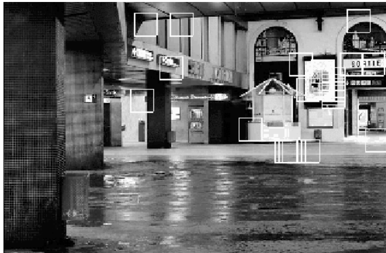
Figure 4.5. The boot-strapping method for training the SVM based face detector. The false positive detections are marked with white boxes.
