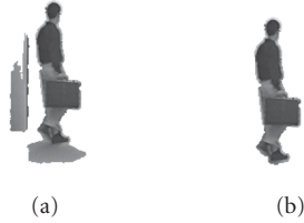
FIGURE 5: Comparison of results from the test sequence Hall Monitor. The binary change detection mask is superimposed on the original image. The results of the classification (a) is refined by the post-processing (b) to eliminate the effects of shadows.
