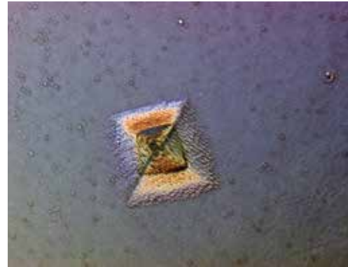
Figure 22. Mechanical testing of human dentine using an indenter. Field width 600 µm.
