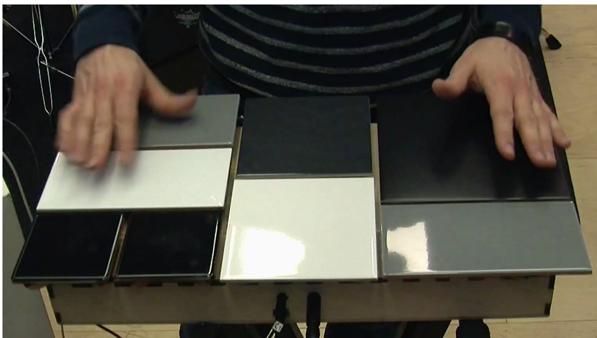
Figure 1. The instrument built from eight ceramic tiles with piezo discs attached to them to sense vibrations.
