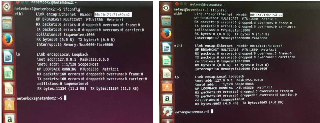
Figure 4.12: The network configuration of NetEmBox with one Network Interface Card (NIC) left, and network configuration with two NICs after the upgrade, right.
