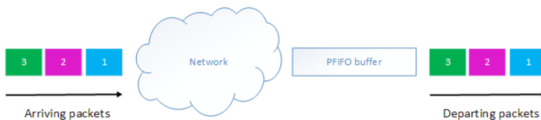
Figure 3.9: A PFIFO queue, which resembles a voice circuit network where packets are in order on the receiving end
