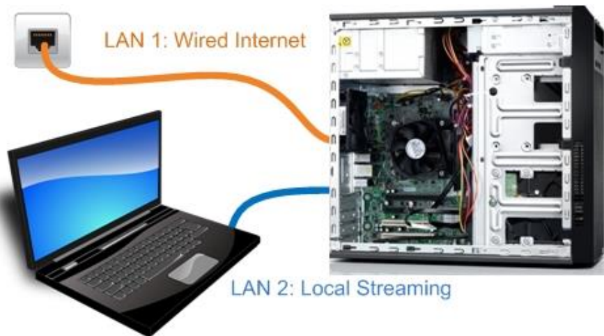
Figure 4.13: NetEmBox-1 upgrade – separate LAN ports for a wired Internet connection and local streaming
