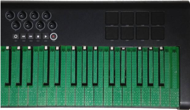
**Figure 4.** Capacitive touch sensors on a MIDI keyboard.
