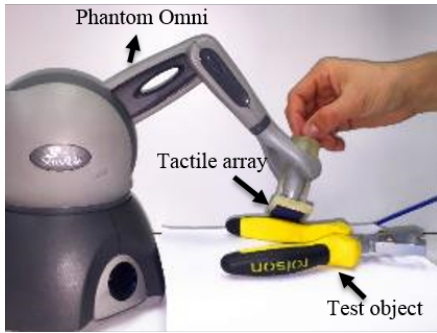
Fig. 2: A Phantom Omni device is used as a robotic arm to explore the object and a tactile sensor is attached to its stylus.
