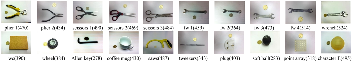
Fig. 3: Objects used for the experiments, labeled from 1 to 20 (left to right, top to bottom). The name and number of collected tactile readings are also given below each object. Note: fw and wc stand for fixed wrench and wooden cuboid respectively.
