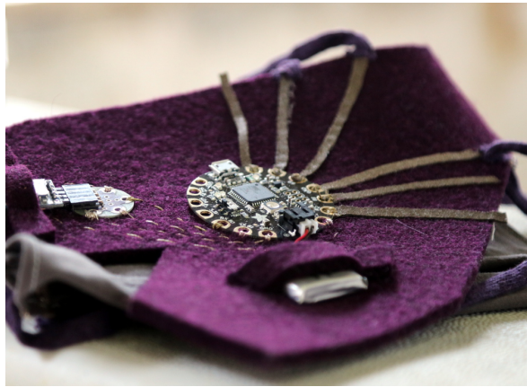
Figure 2. Adafruit Flora microcontroller in an e-textile circuit with conductive fabrics and thread. The Flora iterates on the open source design of the Lilypad using the same sewable connections on the PCB.
