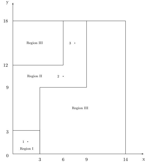
(a) A schematic of the geometry for this dog-leg duct (dimensions in cm). Three nodes numbered 1-3 are referenced in figures below and are located at coordinate points (1.5,1.5), (6,10.5), and (7.5,16).
