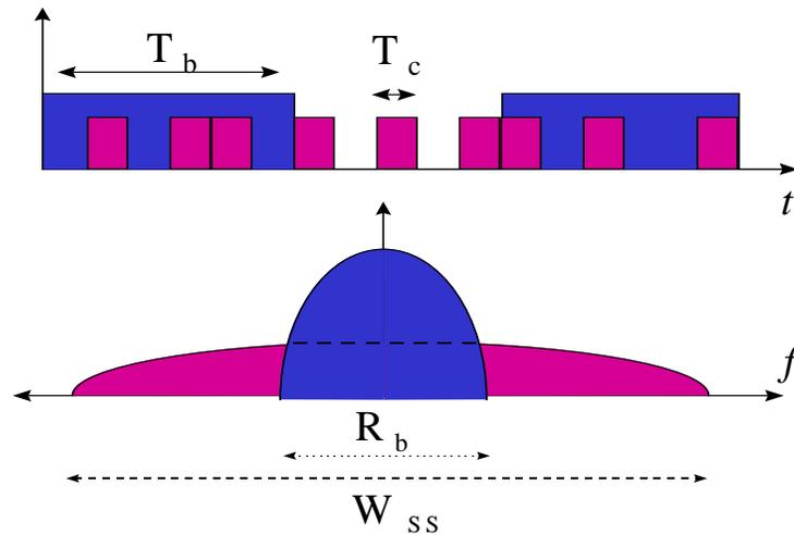
Figure 1.1 Illustration of DS-CDMA spreading and despreading process in time and frequency domain.
