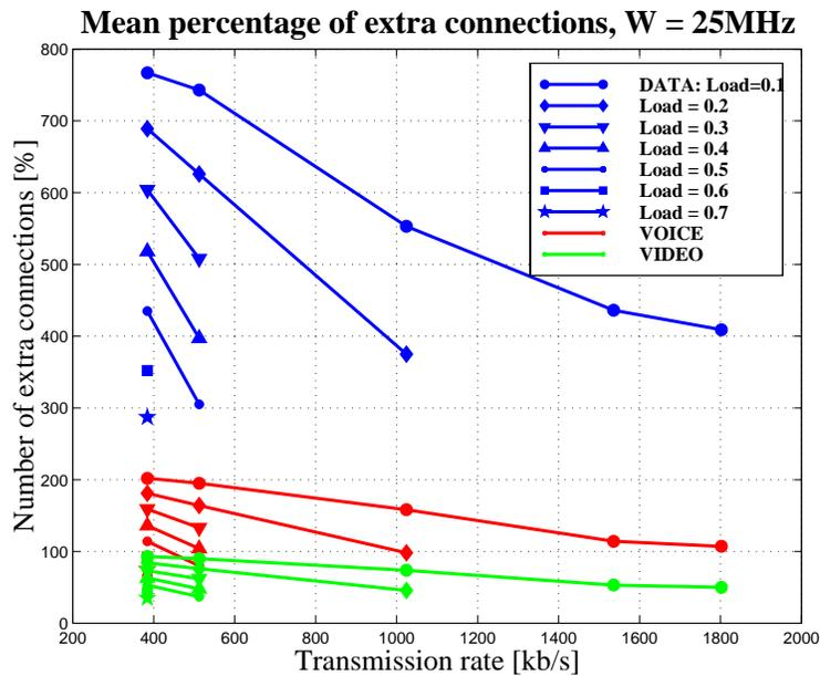
Figure 5.16 Percentage of the highest number of extra voice, video or data connections that could be accepted above the theoretical capacity  $C_{max}$  when channel bandwidth is  $W_{ss} = 25$  MHz.
