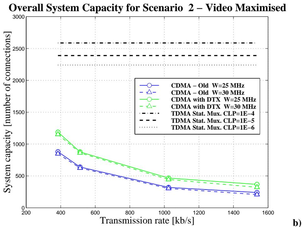
Figure 5.14 System capacity when unused capacity is allocated to only one traffic type: a) voice, b) video. Only values for channel bandwidths  $W_{SS}=25$  and  $W_{SS}=30$  MHz are shown., as all other channel bandwidths yield very similar results.
