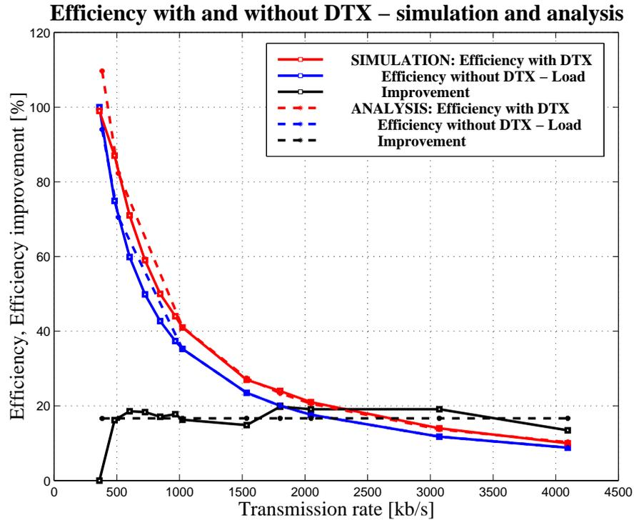
Figure 5.5 Comparison of analytical and simulation results for efficiency and efficiency improvement.
