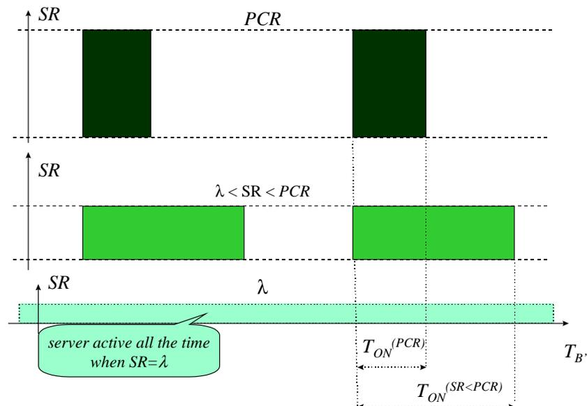
Figure 3.7 Illustration of simulated values of multiplexer slot (i.e. service) rate, and how the slot rate influences the duration of the busy period of the multiplexer.
