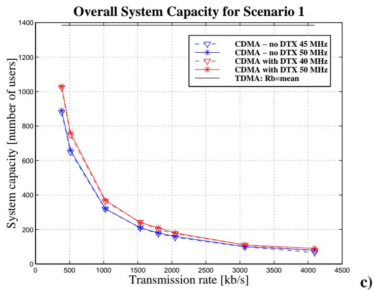
Figure 5.4 Overall system capacity vs. transmission rate  $R$  for various channel bandwidths  $W_{ss}$ , and comparison to TDMA when data rate is equal to the mean rate ( $R_d = \lambda$  [kb/s]):
