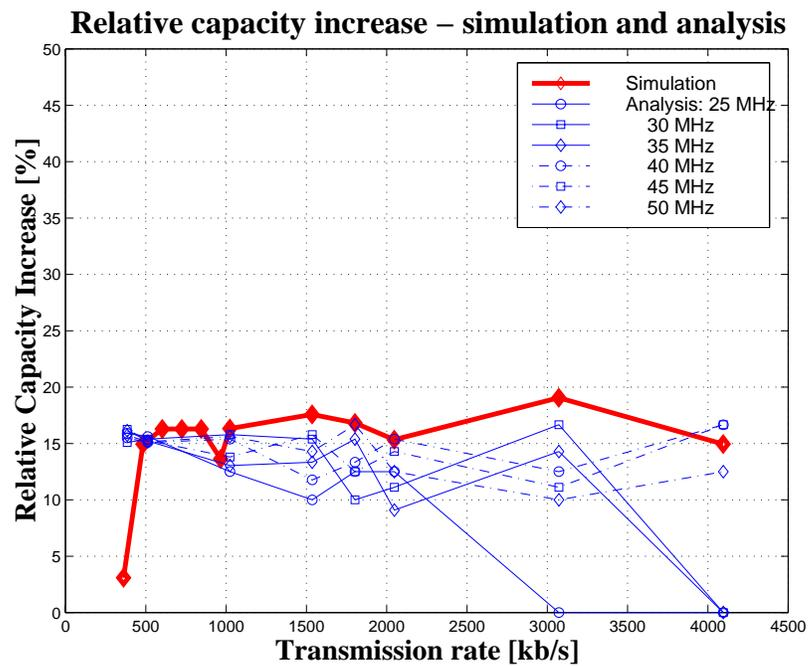
Figure 5.3 Relative capacity increase vs. transmission rate. The thin blue lines represent analytic results for various channel bandwidths.
