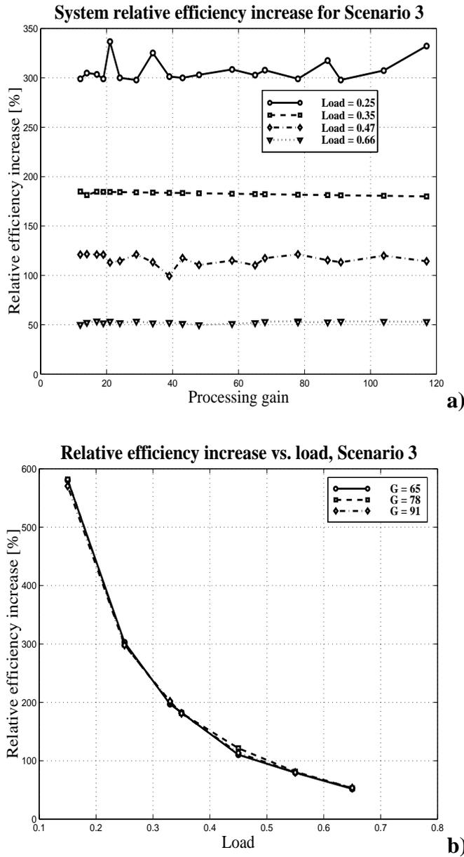
Figure 5.27 Relative efficiency increase obtained with DTX vs. a) processing gain and b) load.
