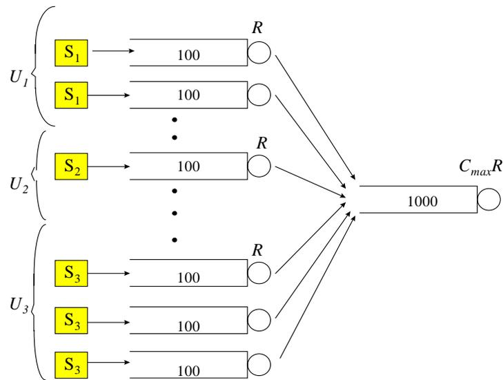
Figure 5.8 Simulated configurations. The notion of “terminal” is not relevant in Scenario 2, as the codes are allocated to VCCs, and thus a terminal can have any number and combination of connections.
