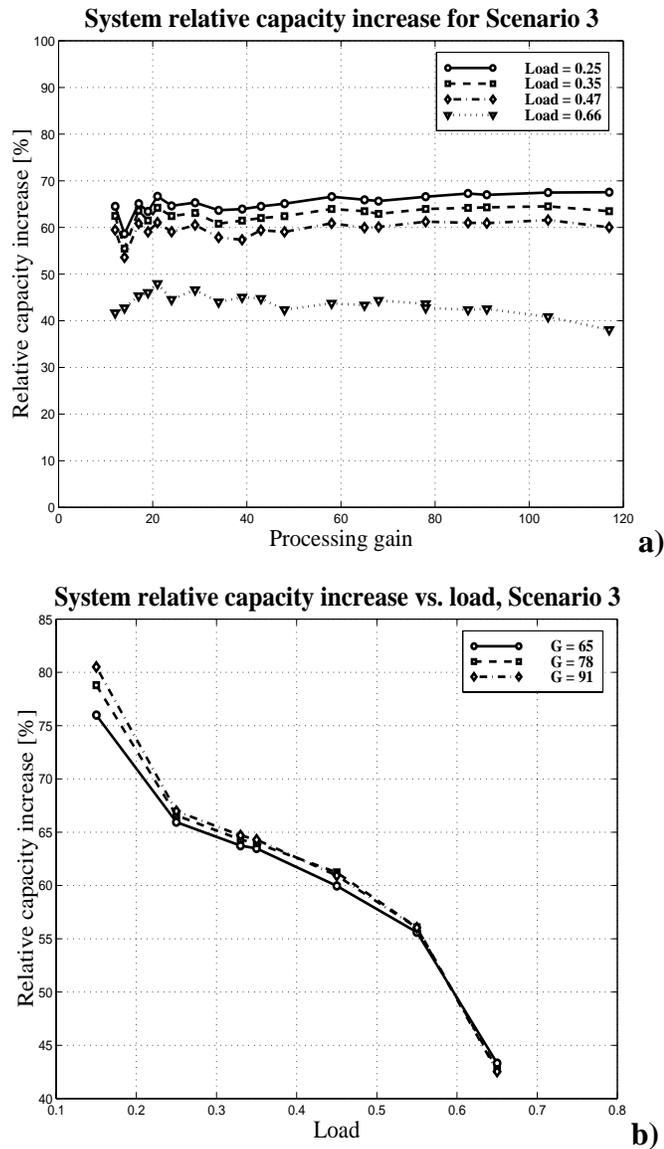
Figure 5.26 Relative capacity increase vs. a) processing gain and b) load.
