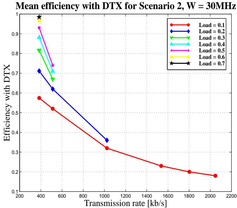
Figure 5.19 Mean efficiency when DTX is employed vs. transmission rate: analytical results for  $W_{ss}=30\text{ MHz}$ .
