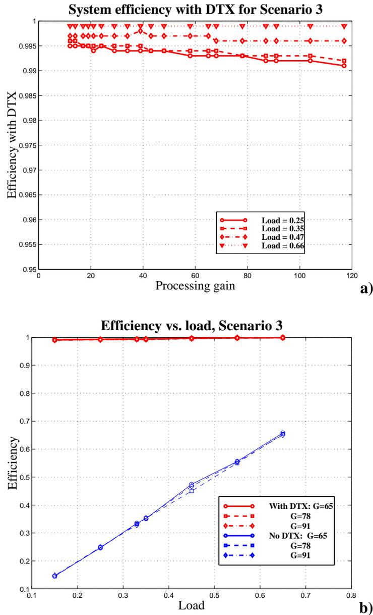
Figure 5.25 Efficiency achievable with DTX vs. a) processing gain and b) load.
