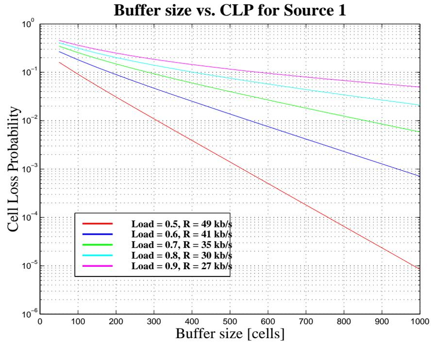
Figure 5.20 Cell loss probability (CLP) versus buffer size, for voice traffic.
