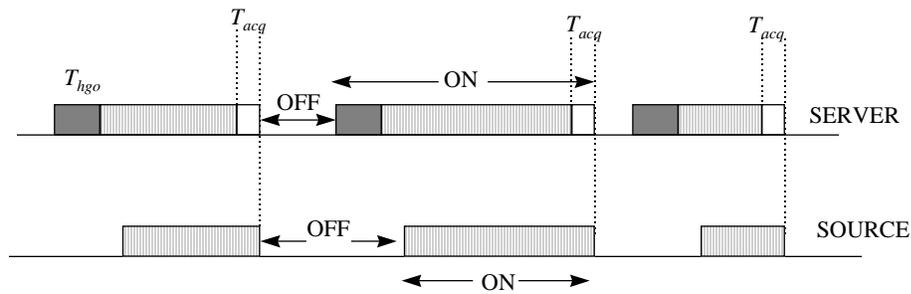
Figure 3.5 Illustration of inserted overhead at the output of the multiplexer, i.e. server.
