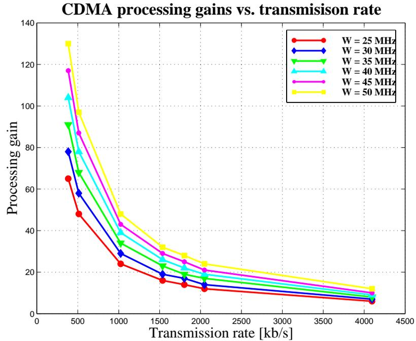
Figure 5.23 Plot of processing gains  $G$  versus transmission rate  $R$  for various channel bandwidths  $W$ .
