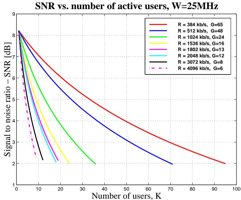
Figure 5.10 SNR versus number of simultaneously active users.
