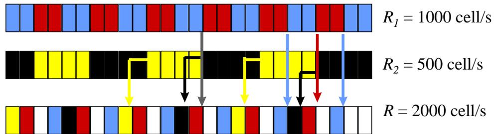
Figure 3.4 Insertion of empty cells between the cells of connection multiplexed streams.  $R_1$  and  $R_2$  are the cell arrival rates of two connections during their active periods, and  $R$  is the transmission or cell slot rate at the output of the multiplexer, i.e. on the uplink. The cells are sent on the uplink after they are fully received in the buffer. The arrows show when the arrived cells are sent in cell slots.
