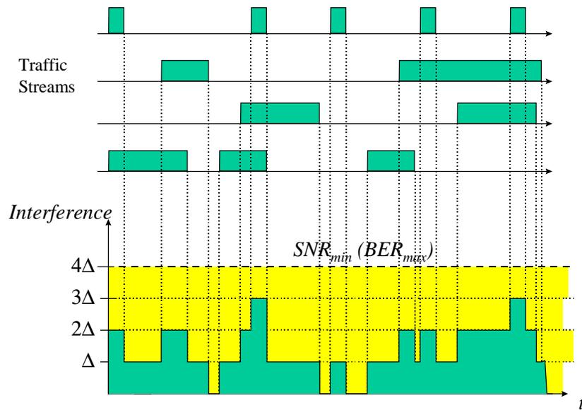
Figure 5.9 Illustration of the interference-limited randomly changing CDMA capacity.
