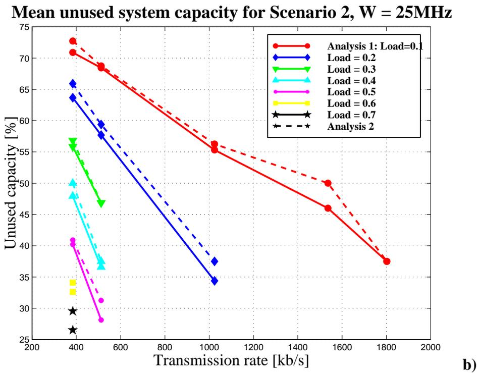
Figure 5.12 a) Busy periods of sources when transmission rate is varied, and b) how these busy periods translate into the mean unused capacity: dotted lines represent the results from the analysis of the p.d.f. of the mean number of active users at any one time for channel bandwidth of 25 MHz.
