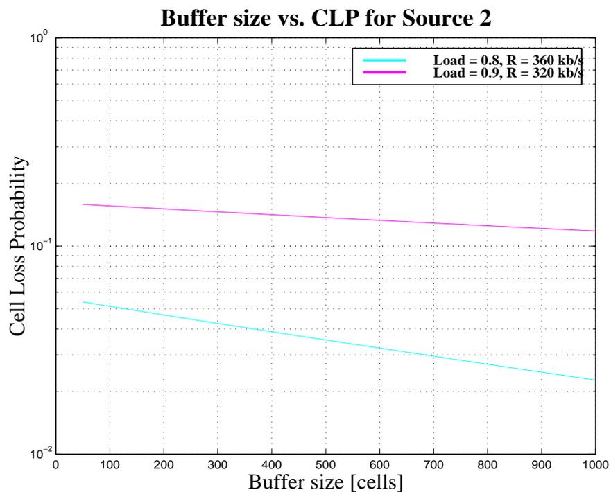
Figure 5.21 Cell loss probability (CLP) versus buffer size, for video traffic.
