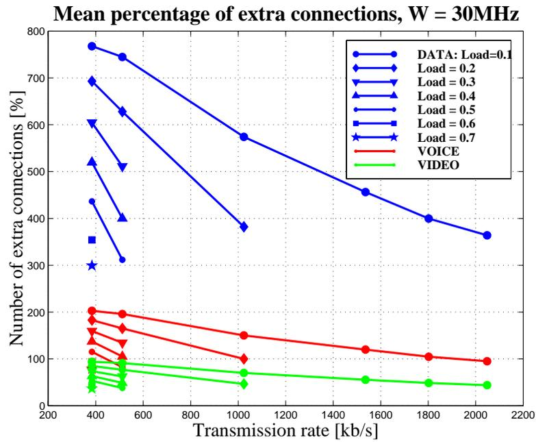
Figure 5.17 Percentage of the highest number of extra voice, video or data connections that could be accepted above the theoretical capacity  $C_{max}$  when channel bandwidth is  $W_{ss} = 30\text{MHz}$ .
