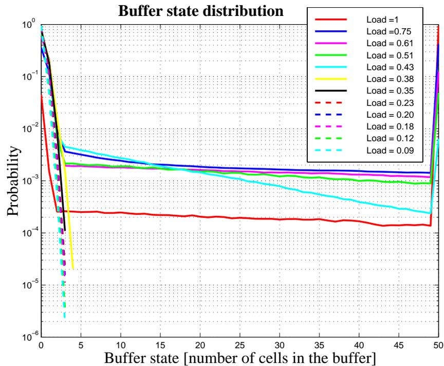
Figure 5.6 Buffer state distribution - simulation.
