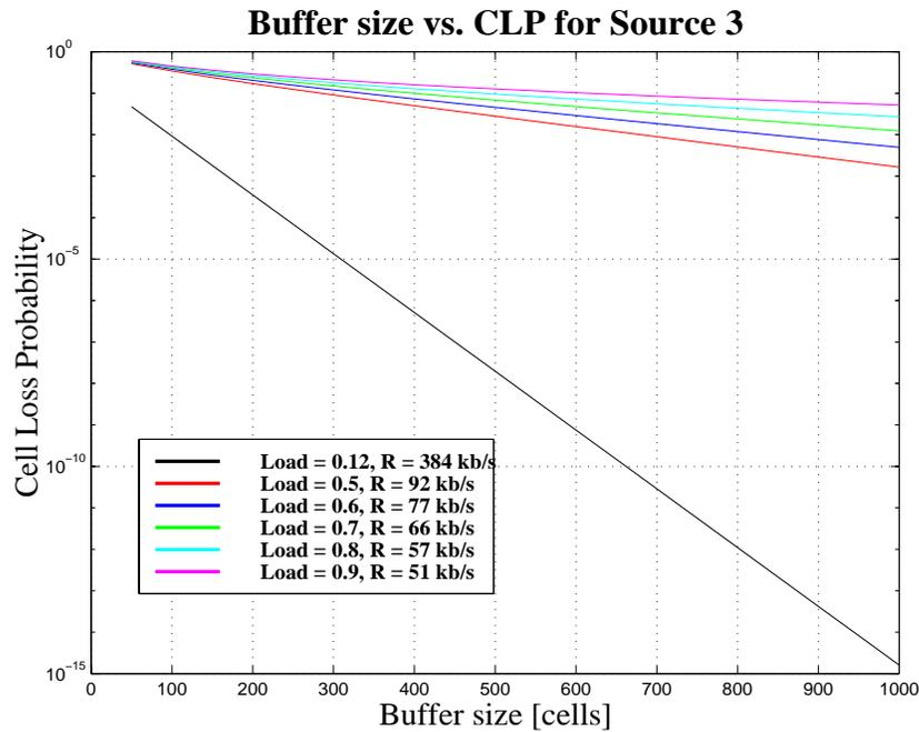
Figure 5.22 Cell loss probability (CLP) versus buffer size, for data traffic. The black line is the plot for  $R=384$  kb/s, the only critical transmission rate of those examined for data traffic.
