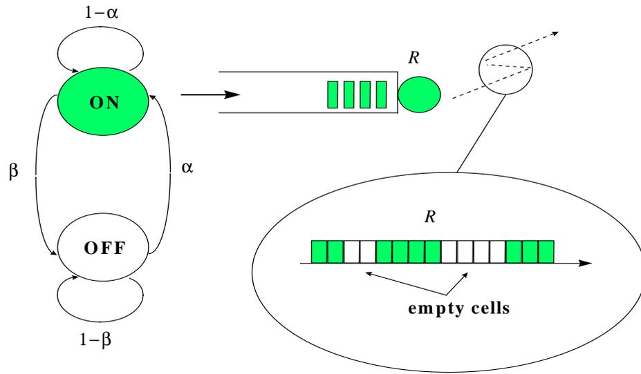
Figure 3.6 Modelling of a source, multiplexer, and cell stream on the uplink.
