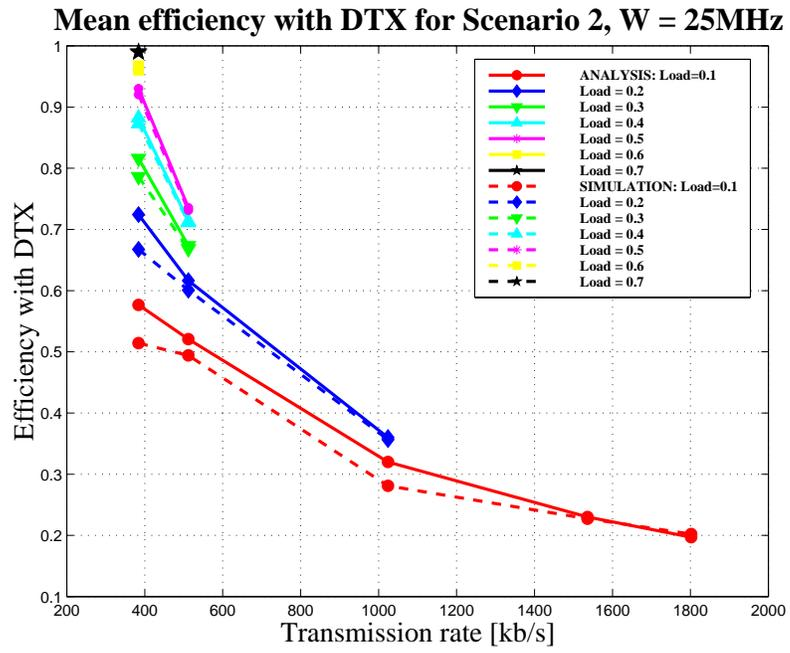
Figure 5.18 Mean efficiency when DTX is employed vs. transmission rate: comparison of analytical with simulated results for  $W_{ss} = 25\text{ MHz}$ . . All broken lines on graph are simulation results.
