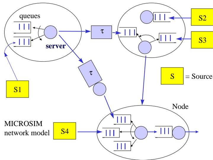
Figure 4.1 MICROSIM network model: nodes comprise input queues, zero-delay switch, node delay element that models switching delay in the node, and output queues. A node must have at least one input queue. Delay on transmission links is modelled using a delay element, but links may have zero delay.
