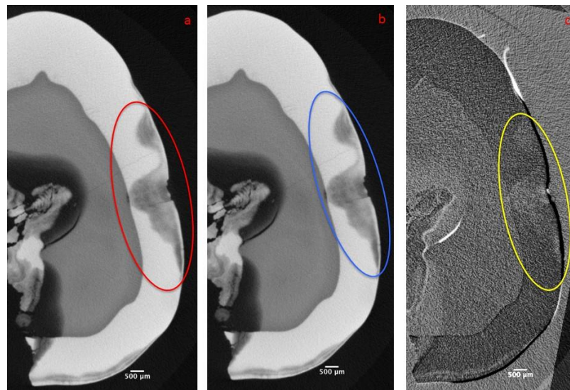
Figure 10.9 XMT images of Br20A: (a) before, (b) after infiltration. (c) Subtracted XMT image (contrast adjusted) showing the higher grey values (an indication of infiltrated radiopaque material in the lesion). The circles show the lesion.
