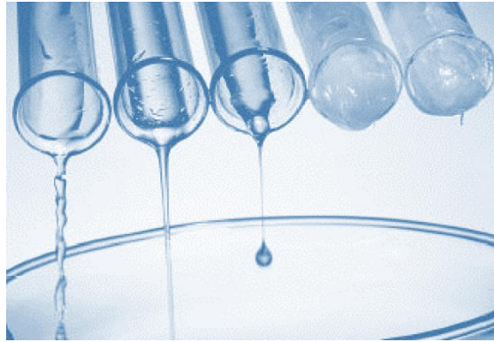
Figure 9.2 Viscosity is the resistance of the liquid to the deformation. This image is (left to right) showing an increase in viscosity of the liquids ( http://www.synlube.com/viscosity.html , accessed on 21/02/2017).
