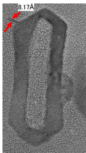
Figure 3.10 TEM image of enamel crystal showing dissolution at the centre of the crystal (Yanagisawa and Miake 2003).
