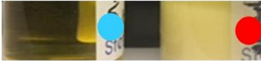
Figure 8.1 Showing the homogenous (bottle with the blue dot) and agglomerated (bottle with the red dot) consistency of samples.
