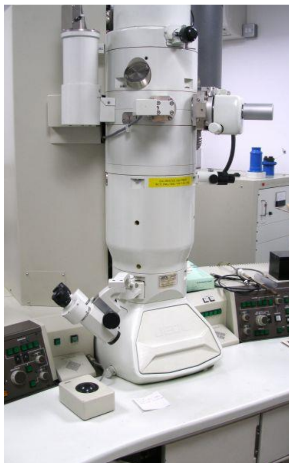
Figure 14. TEM microscope JEOL 2010: high resolution TEM operating at 200kV, lattice image resolution to 0.15nm, provided by NanoVision.
