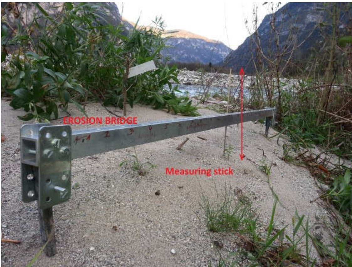
Figure 7.4 Photograph of the erosion bridge and measuring rod (used for measurement of elevation).
