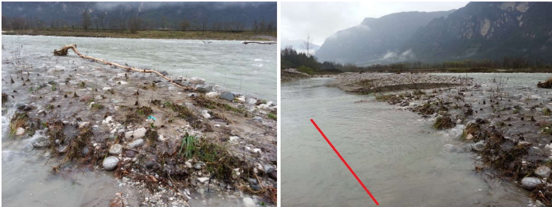
Figure 7.15 Site eight after a major flood event. Left photo shows the top of the mid channel bar. The red line in the right photo indicates original position of bank and transects.
